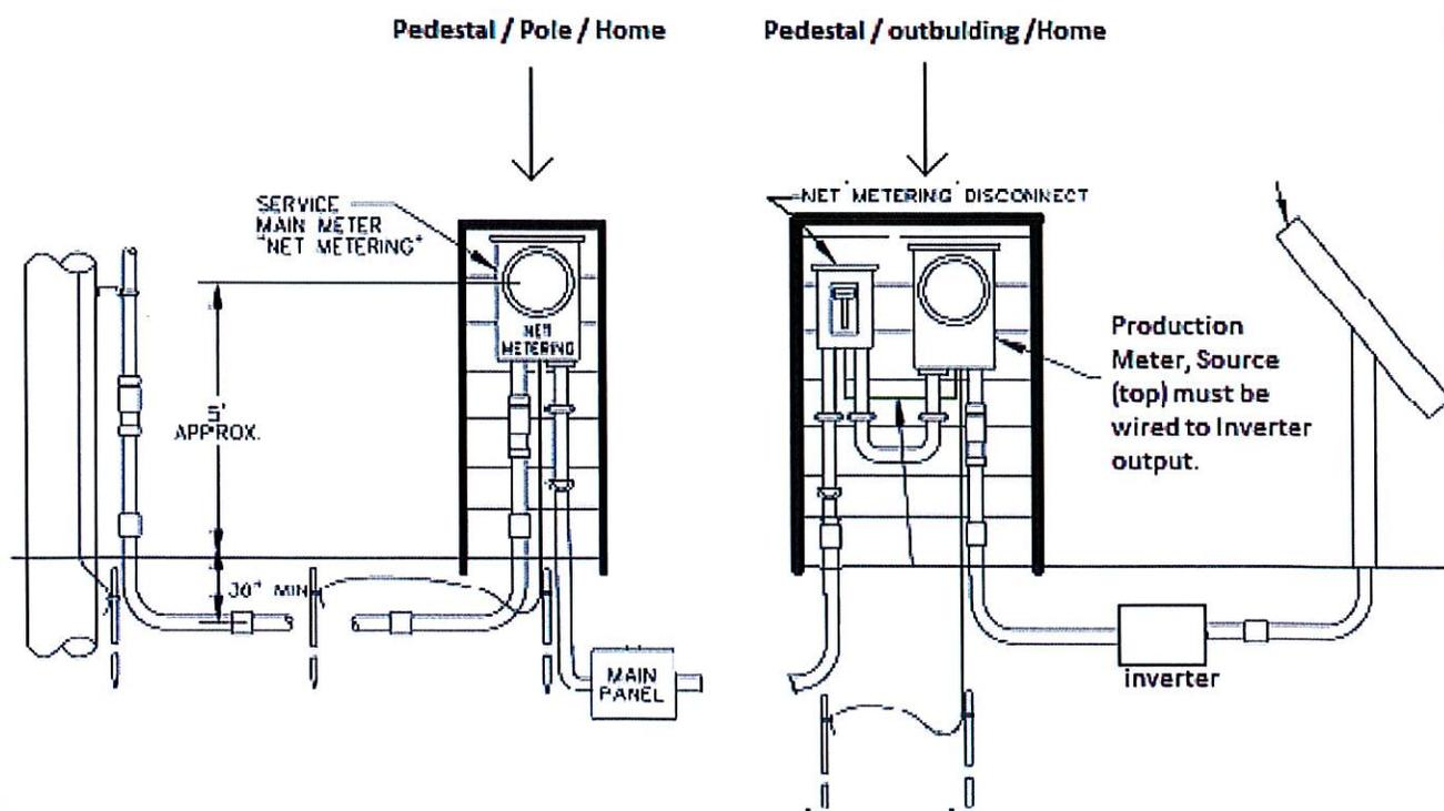
**Grounding for this type of installation: The Main Service Meter base and the Solar Production Meter base will have separate grounds, Grounds will consist of two electrodes bonded together and separated by at least 6 feet at each Meter base, the ground from the Solar Production Meter Base will be extended to the disconnect switch with #6 Copper. See the above referenced drawing.**
